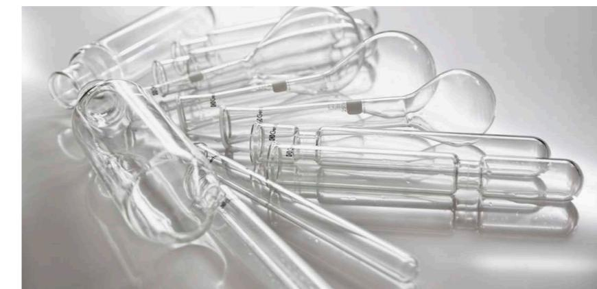
Digestion tubes and Kjeldahl flasks
